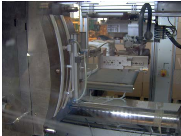
Fig. 4. The machine for injecting plastic materials.
